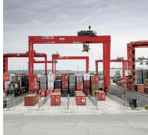
Automatic stacking crane
