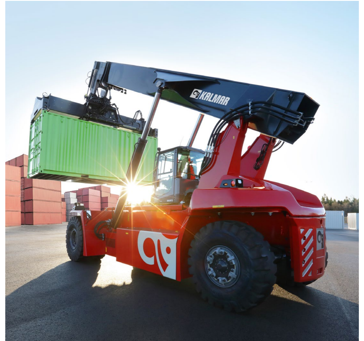
Innovation example: In December, Kalmar launched three 100% electric-powered solutions. The electric reachstacker was one of them.
