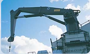
Marine Deck crane
