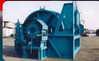
Mooring winch system
