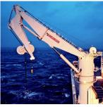
North Sea Shipping North Sea Giant, one of the world's largest offshore construction ships, features a 400-tonne MacGregor crane. More...
